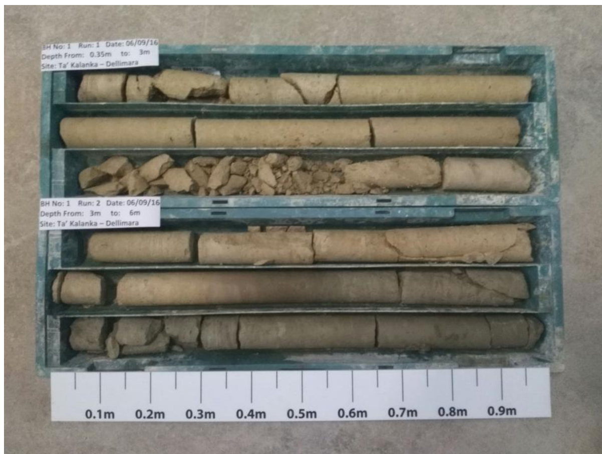
Plate 1: Photograph of core sample recovered from BH1 Run No.1 and No.2
