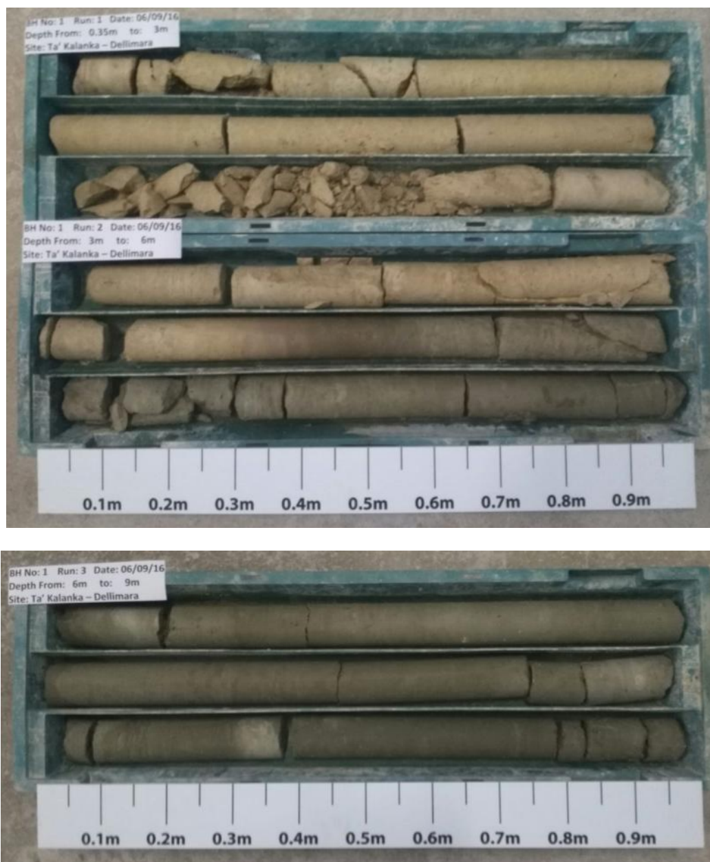
Figure 18: Photographs of the core samples recovered from BH1 during ground investigation. Fractured rock is mainly due to mechanical damage
